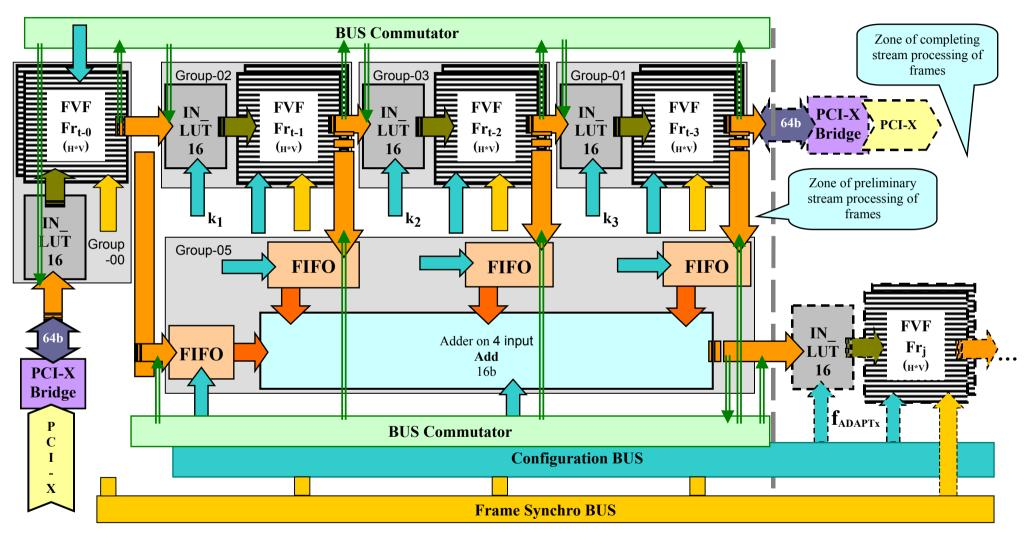
The total delay in a zone of preliminary frame stream processing, if bypassing FE  $Add_3$ , makes one frame, due to recording of the initial frames maps to FE FVF -  $Fr_{t-0}$ . Indexing t-0 ... t-3, instead of i, j, .. is applied for comprehension of conveyor operation the with stream of frames created in miscellaneous instants.
