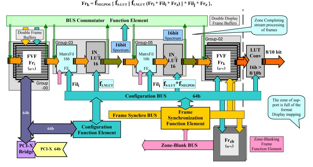
The total delay in a zone of final frame stream processing of, bypassing FE FVF -  $\mathbf{Fr}_k$ , makes 2 frames, due to recording of the initial frames to FE FVF -  $\mathbf{Fr}_i$ . For simplification is not rotined FE IN\_LUT16 on an input FE FVF -  $\mathbf{Fr}_i$ .
