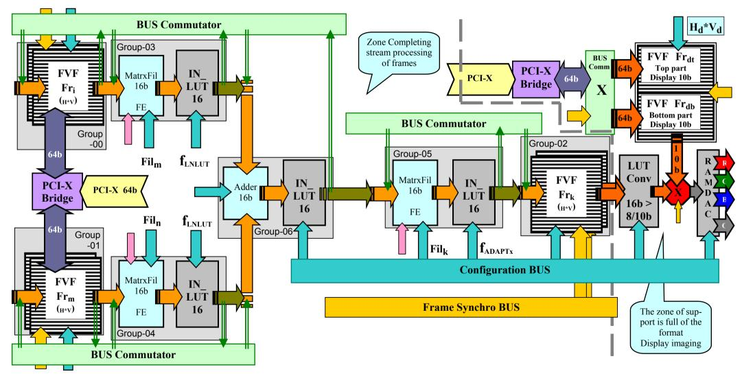
The total delay in a zone of final frame stream processing, bypassing FE FVF -  $\mathbf{Fr}_k$ , makes 2 frames, due to recording of the initial frames maps to FE FVF -  $\mathbf{Fr}_i$  and FE FVF -  $\mathbf{Fr}_m$ . For simplification are not rotined FE IN\_LUT16 on inputs FE FVF - Fri and FE FVF -  $\mathbf{Fr}_m$ .
